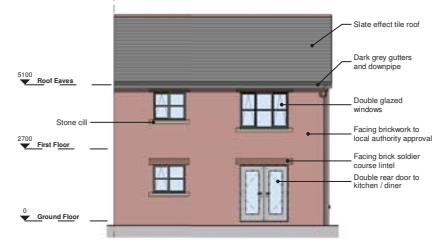
5 Rear Elevation_Brick Scale: 1 : 100
